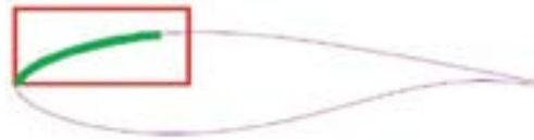
FIGURE 2. Airfoil high fidelity computational domain within the rectangle, heater covers green area
