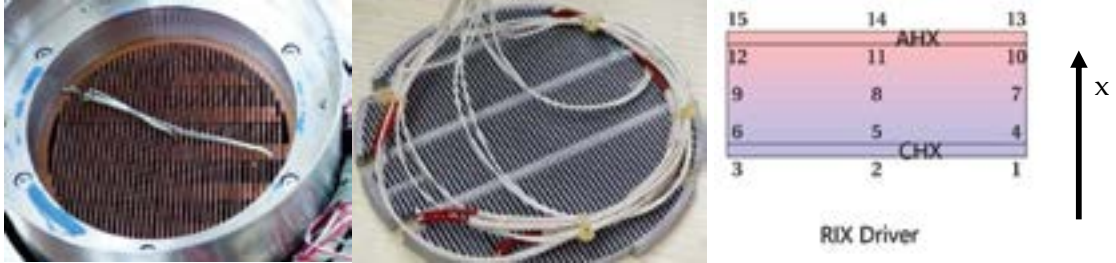
FIGURE 3. From left to right: Ambient heat exchanger (AHX), cold heat exchanger (CHX), and thermocouple positions
