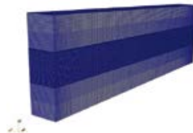
FIGURE 2. Computational grid employed for numerical simulations, composed of 1,348,800 cells
