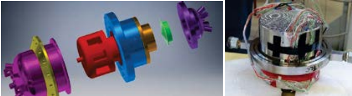
FIGURE 1. Exploded view of the TACOT and photo of its core
