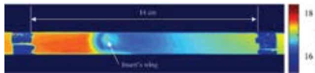
FIGURE 3: A representative infrared image: butterfly insert - Re = 5030 .
