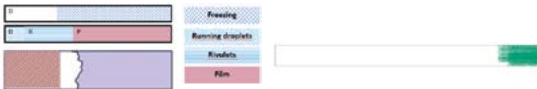
FIGURE 3. Hydrophilic surface: top left trace of frozen beads, middle left, water regimes from simplified model; bottom left, iced area derived from [10]. Right: high fidelity iced bead traces
