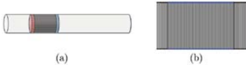
FIGURE 1. (a) Simulated standing wave device. (b) 1D Mesh of the stack.
