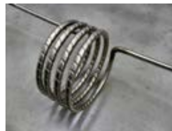
FIGURE 9: A section of the coiled wall corrugated tubes tested.
