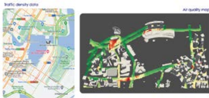
FIGURE 8. Air quality prediction for a given wind and traffic conditions
