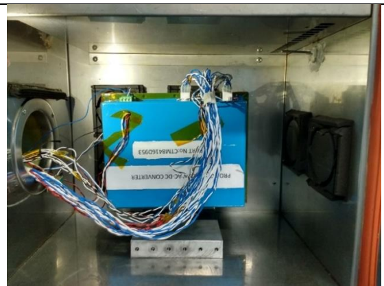
Figure 13. Converter inside the rapid temperature cycle chamber.
