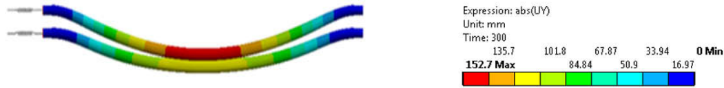
FIGURE 9. Deflection profile at the simulation end time
