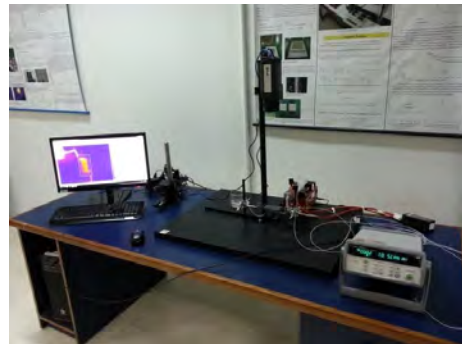
FIGURE 2b. Experimental apparatus for infrared thermography analysis of micro-heat exchanger.
