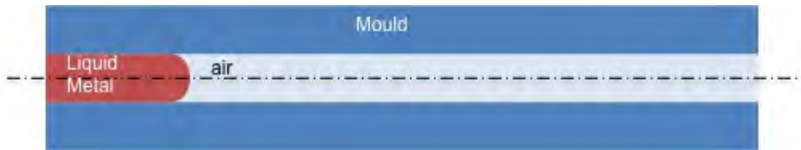
FIGURE 2. Schematic description of the infiltration problem
