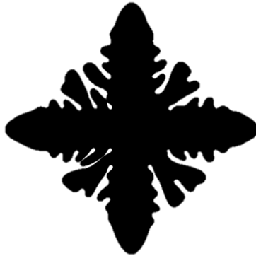
FIGURE 2. Simulated dendrite, grown for 10ms from a melt that is undercooled by 8K; the total length of the dendrite in horizontal and vertical direction, respectively, is 40 \mu m.
