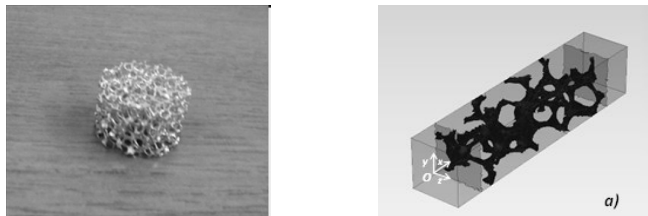
FIGURE 1. Aluminum foam: a) sample; b) RVE extracted from the CT data.
