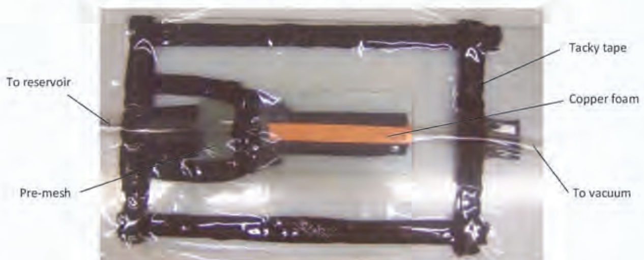
FIGURE 2. Copper foam inside the experimental set-up.
