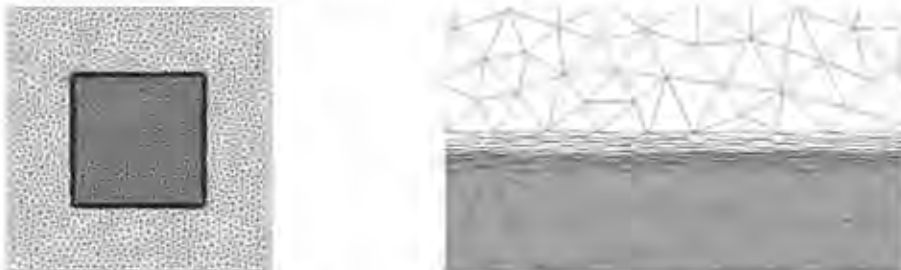
FIGURE 1. Mesh adaptation process from an isotropic distribution to an adapted anisotropic mesh in the vicinity of the interface.
